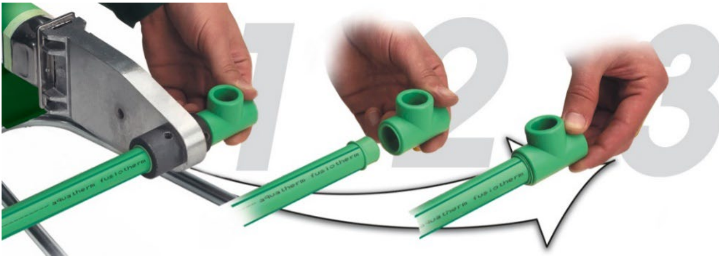
Basic fusion steps: 1. Heat 2. Press 3. Cool
